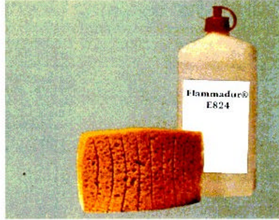
Expanded swell module after soaking with impregnation liquid E824. The volume expands up to ten times the original size.
